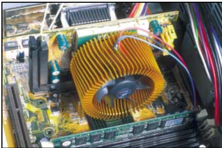
My humble Asus P2B motherboard keeping it real: the Iwill Ssocket can handle FC-PGA CPUs and instruct the Asus to supply a lower voltage. Here I've got a PIII overclocked to 1GHz on a 133MHz FSB, with the help of PC133 SDRAM. Note the string used to keep the Ssocket from leaning over the overclocked BX chipset in the absence of any Slot 1 retention guides. Blue Peter eat your heart out! The Titan fan attached to the chip is now available in the UK from Hills Components: www.hillscomponents.co.uk (01923 424344)
